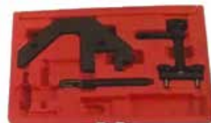
Engine timing tool set for BMW M47
