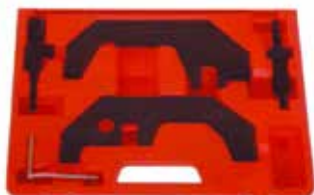
Engine timing tool set for BMW M62/ N73
