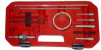
Engine timing tool set for CITROEN/ PEUGEOT
