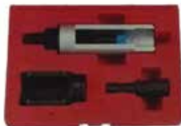
Injector nozzle extractor with spindle
