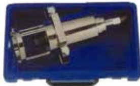
BENZ (W140) Lower control arm bushing remover / installer
