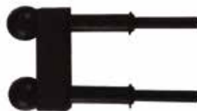
Camshaft locking tool for VW
