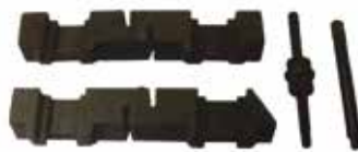
BMW (M60, M62) Camshaft alignment tool
